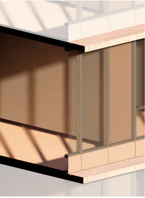
Section 2 Typical window with spandrel
