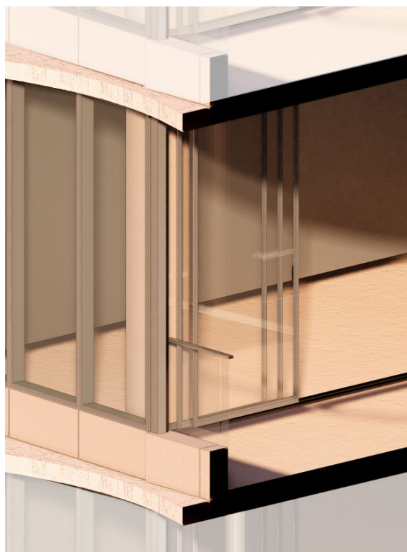
Section 1 Typical balustrade with spandrel
