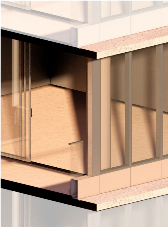
Section 1 Typical balustrade with spandrel
